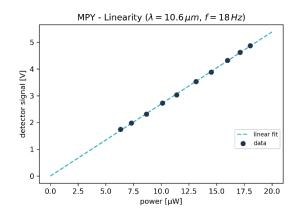
The responsivity and  $D^*$  values are measured with a 150°C blackbody emitter with 6.8 µm peak emission and with a detector with silicon window. The values can change for other wavelengths.
